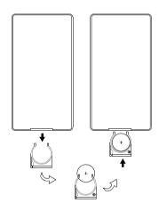
Under normal use the battery will last for about one year. If the remote control unit fails to work even when it is operated near the player, replace the battery. Take out the battery when the remote is not used for a long time.
